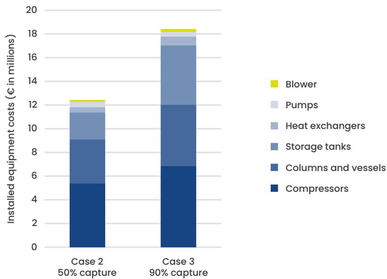
**Figure 5: Total capital expenditure estimates for a 50% and 90% carbon capture system installed on a Suezmax vessel**
