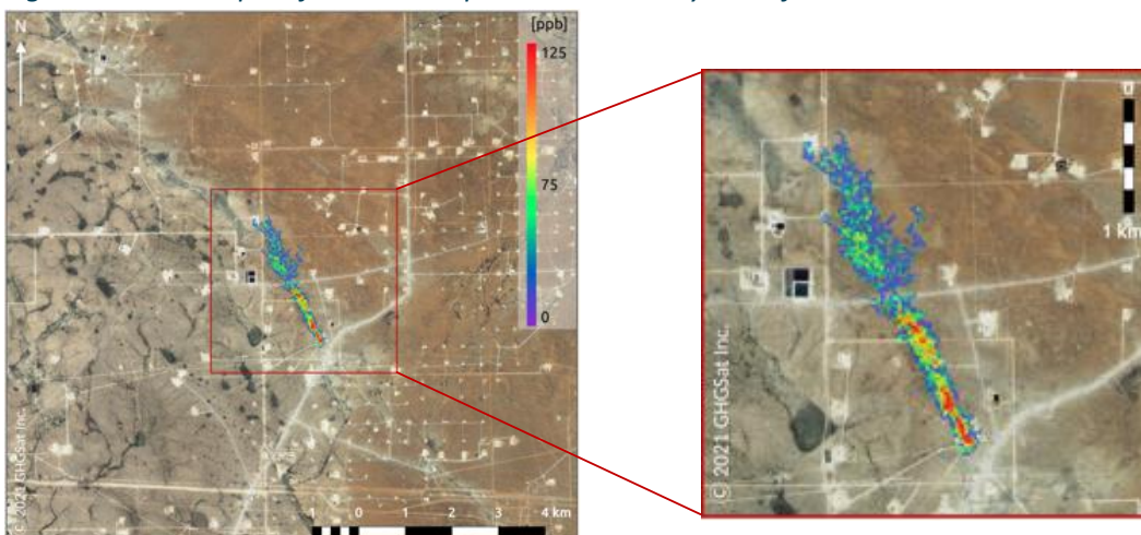
Figure 1: An example of a methane plume detected by one of GHGSat’s satellites over the Permian Basin
