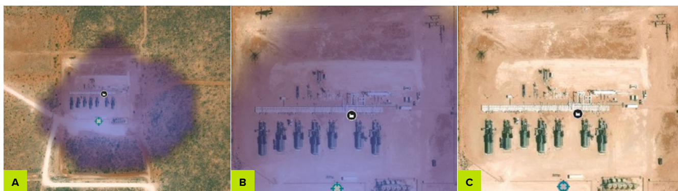
FIGURE 1. Plume image overlay on visual imagery provided by the commercial satellite provider to the operator. Panel A shows the entire plume extent. Panel B zooms in on the area of the plume enhanced in methane and near the identified source of the plume (turquoise marker). Panel C shows only the visible imagery the possible source location (turquoise marker) without the plume overlay. Here no specific source is the obvious origin of the plume. Visual imagery data from ESRI . Plume images and data points from Carbon Mapper .
