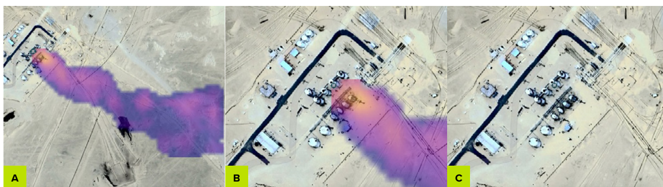
FIGURE 1. Plume image overlain on visual imagery provided by UNEP to the operator. Panel A shows the entire plume extent. Panel B zooms in on the area of the plume enhanced in methane and near the identified source of the plume (turquoise marker). Panel C shows only the visible imagery the possible source location (turquoise marker) without the plume overlay. Here the tanks are clearly visible and are the closest equipment to the detection. Visual imagery data from ESRI . Data points and plume images from UNEP .
